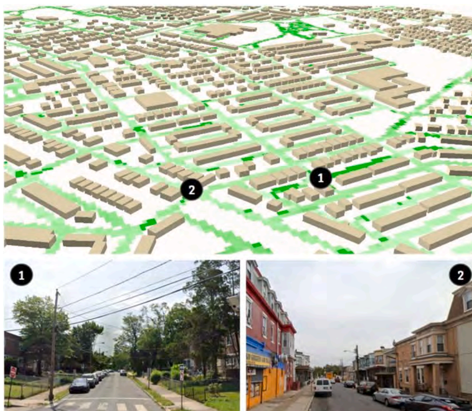
Fig. 5. Examples of streets with high to low VGVI scores in Camden using 3D GIS (represented by darker to lighter green color respectively) and street views.
