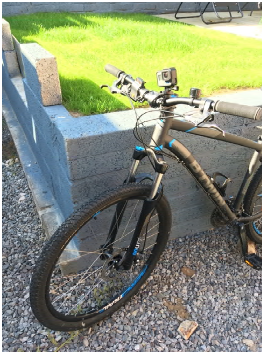
Figure 2. Bicycle-mounted Go-Pro camera on the mounting base that rotates 360° to give different camera angles.
